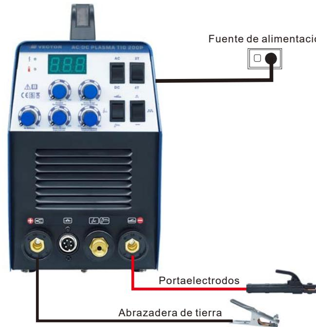
**3.3 Configuración para soldadura HF TIG (GTAW)**
