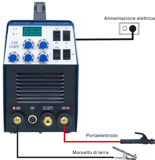
**3.3 Predisposizione per saldatura TIG HF (GTAW)**
