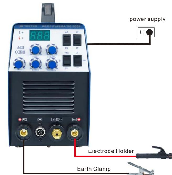
**3.3 Set-up for HF TIG (GTAW) welding**
