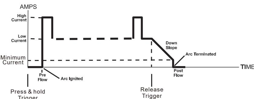
4T Latch mode this mode of welding is mainly used for long welding runs to reduce operator fatigue. In this mode the operator can press and release the torch trigger and the output will remain active. To deactivate the power source, the trigger switch must again be pressed and released, thus eliminating the need for the operator to hold the torch trigger.
